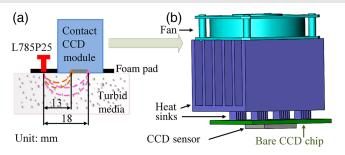
**Fig. 1** (a) A compact DSCF probe placed on the surface of a turbid medium. (b) The DSCF probe consists of a small laser diode (L785P25) and a custom-made contact CCD module, which are confined by a black foam pad and covered by a transparent thin film (not shown) to prevent the CCD sensor/chip from being shortened by the liquid tissue phantom.
