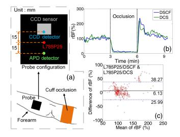
**Fig. 4** *In vivo* experiments on a human forearm to compare the results obtained by DSCF and DCS probes. (a) Experimental setup (bottom) and the configuration (upper) of contact DSCF and DCS probes. (b) Forearm rBF responses during arterial occlusion measured by the DSCF and DCS probes. (c) Bland–Altman plots for the comparisons between rBF changes measured by the two probes.
